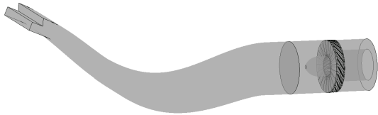
图 3 进气道 S 弯扩压段-压气机一体化模型计算域 Fig. 3 Calculation domain of the integrated finite element model of the inlet S-bend diffuser and compressor
