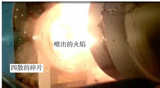
图 32 发动机包容试验时尾喷管出口喷火现象 Fig. 32 Tailpipe flame ejection during engine containment test
