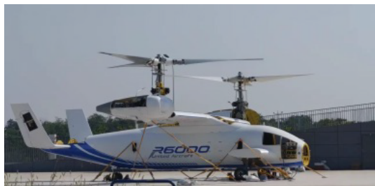
图 33 翎影 R6000 配装 AES100 地面试验 Fig. 33 Ground test of the Lanying R6000 equipped with the AES100 engine
